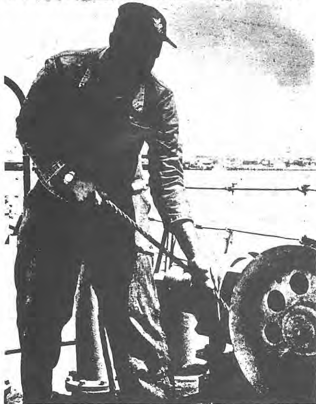
BM/1 William D. Soule operates the capstan which will raise or lower the motor whale boats aboard the Coast Guard Cutter Escanaba. Soule is serving a weekend of ship board augmentation training aboard the Escanaba.
